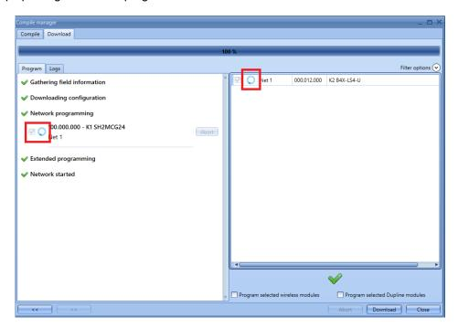
This problem occurs every time a project contains a *Multigate* function that is configured as NAND operator without input signals (the *Input signals* window is empty).
