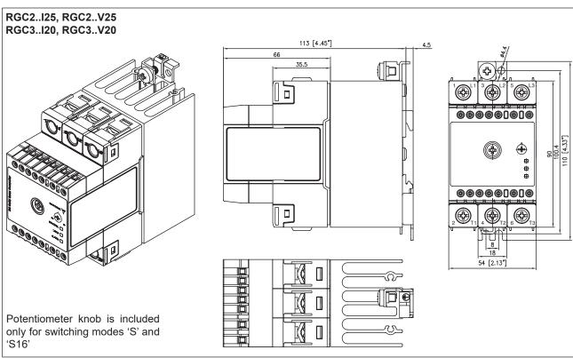
Housing width tolerance +0.5mm, -0mm as per DIN 43880. All other tolerances +/- 0.5mm. Dimensions in mm.
