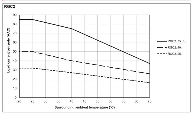
Note: Versions that utilise 24 VAC external supply (Us) are limited to a maximum operating temperature of 60°C (140°F)
