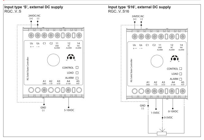
Note: Control input shall be connected to terminals A1-A4 in the case of the RGC3P..S.. In the case of the RGC3P..S16.., the control input shall be connected to either A1-A2 or A1-A3 or A1-A4 or A1-A3-A5 in case an external potentiometer is used.
