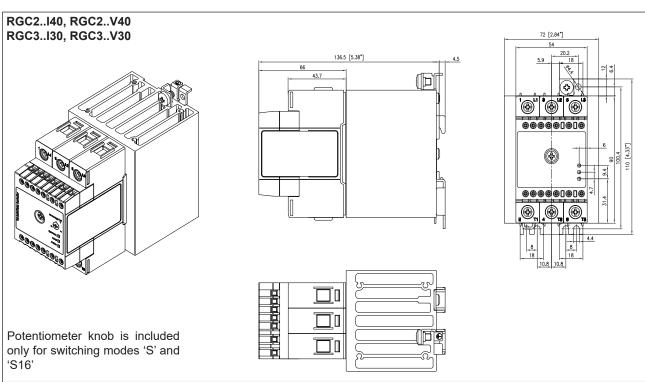
Housing width tolerance +0.5mm, -0mm as per DIN 43880. All other tolerances +/- 0.5mm. Dimensions in mm.
