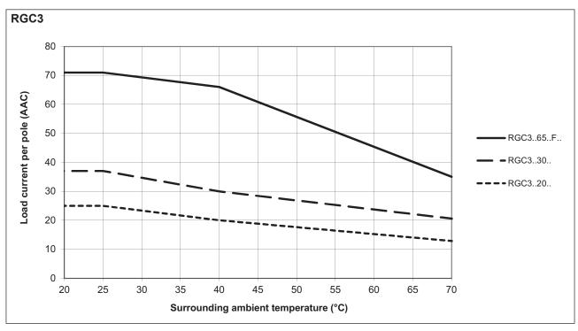
Note: Versions that utilise 24 VAC external supply (Us) are limited to a maximum operating temperature of  $60^{\circ}$ C ( $140^{\circ}$ F)
