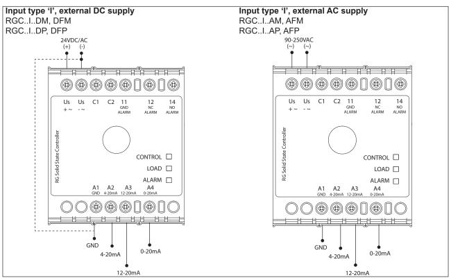
Note: Contol input shall be connected either to A1-A2 or A1-A3 or A1-A4 only
