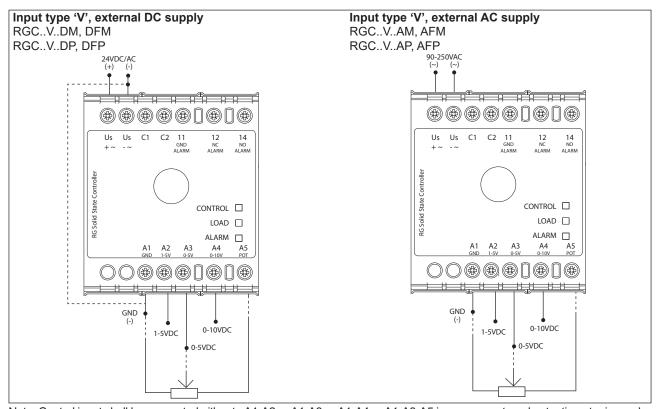
Note: Control input shall be connected either to A1-A2 or A1-A3 or A1-A4 or A1-A3-A5 in case an external potentiometer is used.
