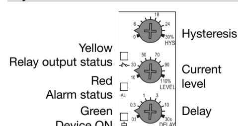
Check if the input range is correct. Turn the power ON. The green LED is ON. Adjust level, delay and hysteresis (difference between the alarm ON and the alarm OFF thresholds) knobs to the desired value. When the input current exceeds (or drops below) the set point for more than the set delay time, red LED (flashing during the delay time) turns ON. Relay and yellow LED turn ON if relay is normally de-energized, they turn OFF if normally energized.
