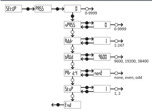
Note: to save the set value, press and hold down the button for about three seconds. To clear changes, wait 20 seconds.
