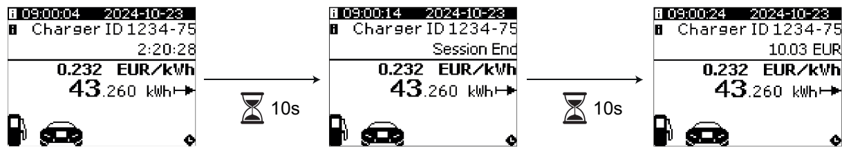
Figure 23 Charging session in progress, with TT field, system power, custom string 1 and 2 active. Time trigger is set to 10 seconds.
