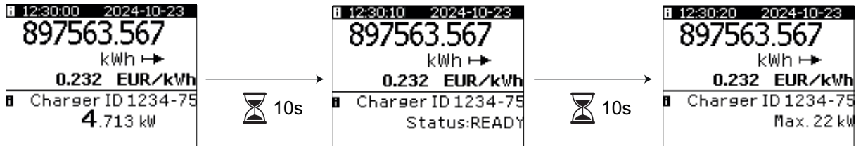
Figure 12 Homepage: page 1 with TT field, custom string 1 and 2 active. rotation time is set to 10 seconds.
