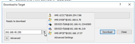
You can even enter the IP address manually or, if available, the host name provided by a DNS server. Using a service tool like Bonjour, Linux-based HMI devices can be discovered using their hostname (e.g., HMI-0d37.local). Bonjour is a trademark of Apple inc.
