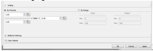
**Scaling** tab converts the tag value. In **By Range** section set the input and output range: the system will automatically calculate the scaling factors.
