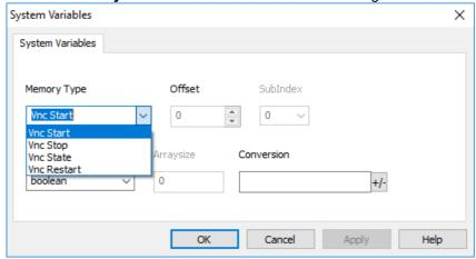
VNC status variables are supported only on Linux devices (See "HMI devices capabilities" on page 539) - BSP version 1.0.344 or greater is required.
