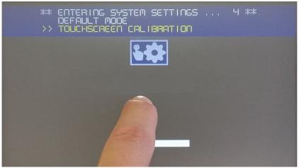
Follow the instructions on screen to complete the calibration procedure, system will prompt to touch specific points to calibrate the touchscreen device.
