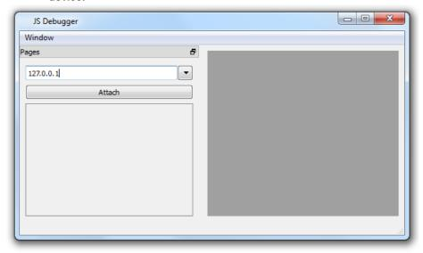
Remote JavaScript debugger connects to BTM-HMI-RUNTIME using port 5100/TCP.
