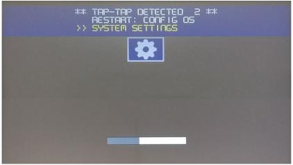
Press on touch screen, "Touchscreen calibration" voice will be highlighted in yellow, hold pressed for few seconds until touchscreen calibration procedure starts
