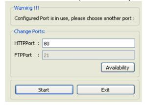
Make sure that when you change this port you also change the port used for download to HMI device in BTM-PC-IDE.
