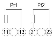
Fig. 11 Temperature inputs 1 and 2 (2 wires)
