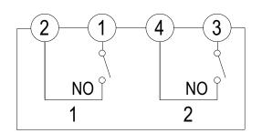
Fig. 10 Digital outputs 1 and 2
