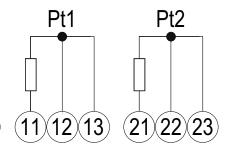
Fig. 12 Temperature inputs 1 and 2 (3 wires)
