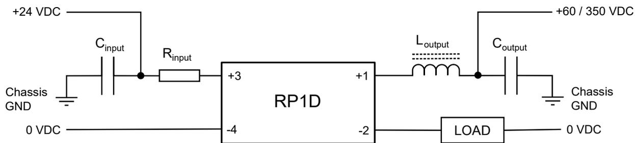
$C_{input} = 1 \text{ nF } 2 \text{ kV (Y2 class, ceramic disc)}$
