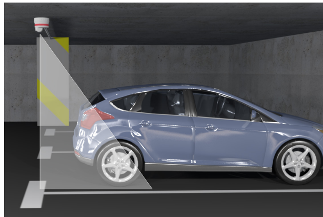
Put the SBPBASEB as close as possible to the parking bay
