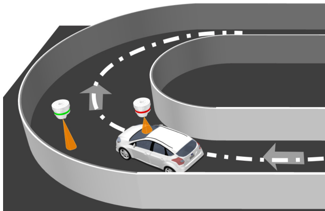
One of the SBPBASEB together with the sensor has been placed too far from the middle of the lane
