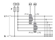
**Fig. 8** One-phase system, six single-phase circuits.
