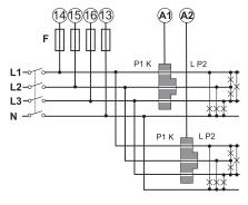
**Fig. 3** Three-phase system, one three-phase circuit.
