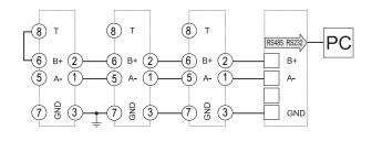
**Fig. 13** Double RS485 port for daisy chain connection.
