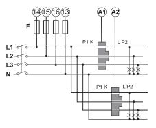
**Fig. 6** Three-phase system, six single-phase circuits.
