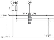
**Fig. 7** One-phase system, three single-phase circuits.
