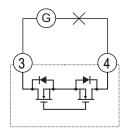
**Fig. 9** Example of connection of multiple EM270s in cascade.
