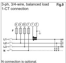
**NOTE**: in the calculations, it is considered only the voltage relevant to L1
