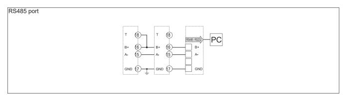
**RS485 NOTE:** additional devices provided with RS485 are connected as per the picture above. The termination of the serial output is carried out only on the last instrument of the network, by means of a jumper between (B+) and (T).
