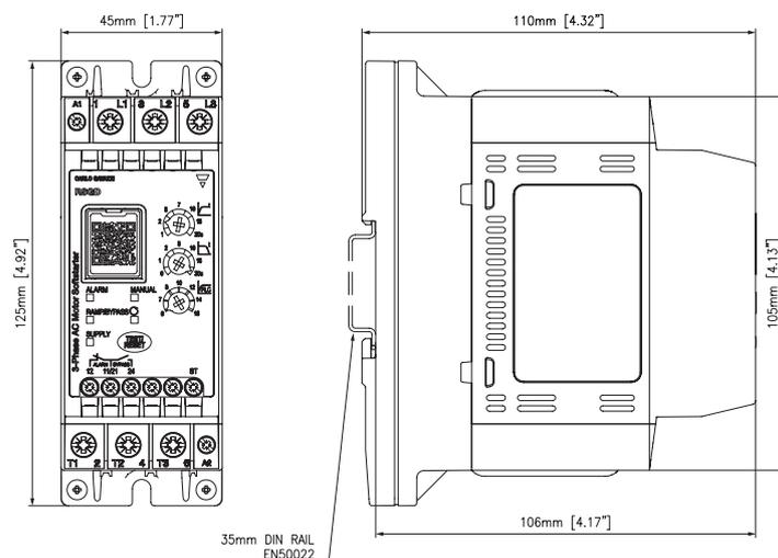
Fig. 1 RSGD..12..VD200 至 RSGD..32..VD200 · RSGD..12..VD210 至 RSGD..16..VD210
