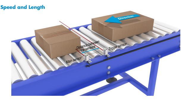
Monitor the speed and length of an object on a conveyor for e.g. sorting on size.
