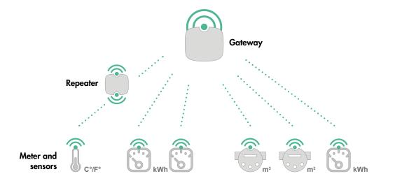
A wireless M-Bus network architecture is made up of the following components:
