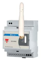
The gateway/receiver offered by Carlo Gavazzi is SIU-MBM-02, which is able to integrate up to 20 wired devices and 32 wireless devices and can transmit data via Modbus TCP/IP (Ethernet port).
