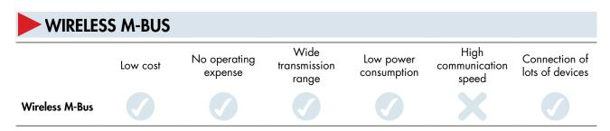
Wireless M-Bus allows transmission up to 100 m in typical applications and this limit, even if it may be reduced in case of concrete walls to 20-30 meters, can still be increased using one or more repeaters. The maximum communication speed is low compared to other wireless technologies, but suitable to transmit consumption and real time data in monitoring applications.
