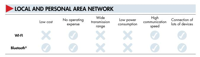
Most local and personal area network technologies, such as WI-FI and Bluetooth<sup>®</sup>, are not suitable for monitoring applications, due to limitations in transmission range typically around 5-10 m. WI-FI could be an option when a suitable number of hotspots is already available (for instance in a commercial building). However, this opportunity is rarely seized because of network access restrictions to internal LANs (for cybersecurity policies) and limited reliability of public networks.
