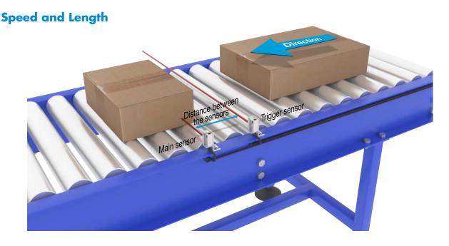
Monitor the speed and length of an object on a conveyour for e.g. sorting on size.
