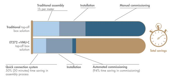
**ET272 +VMU-C tap-off box solution:** no manual configuration, no ID addressing, a general process improvement. Leading to a total configuration and commissioning time reduction from 34 hours of Professionals work to only 2 hours!
