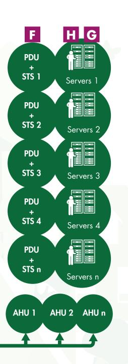
PDU: Power Distribution Unit STS: Static Transfer Switch AHU: Air Handling Unit
